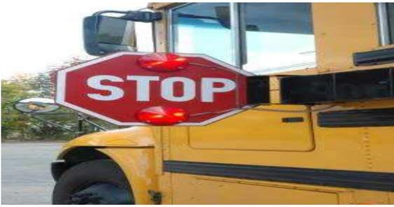
flashing **red lights** indicate the bus **is** loading or unloading.
